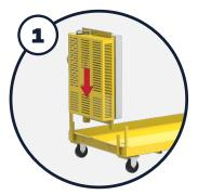
Attach the HEPANOMAD to the platform using the provided bolts (HepaZone SW)
